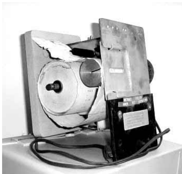
Fig. 11 – An early apparatus for studying verbal learning at the University of Missouri-Columbia, where John A. McGeoch was Chairman from 1930 to 1935. An electric motor advanced the paper roll at preset intervals so that the current trial's stimuli were visible through the slot-shaped window in the metal plate shown here on the right. McGeoch (1932) advanced the idea that forgetting cannot be attributed to the passage of time
