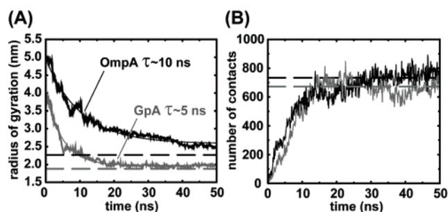
**Figure 2.** (A) Radius of gyration versus time for detergent molecules in self-association simulations. Exponential fits (thin lines) yielded rate constants of 4.9 ns for GpA and 10.4 ns for OmpA. (B) For the self-association OmpA simulation, detergent–protein interatomic contacts (within 0.4 nm) for DPC tails (black lines) and headgroups (gray lines). In both (A) and (B), the respective average values from the last 10 ns of the preformed micelle simulation are shown (horizontal dashed lines).
