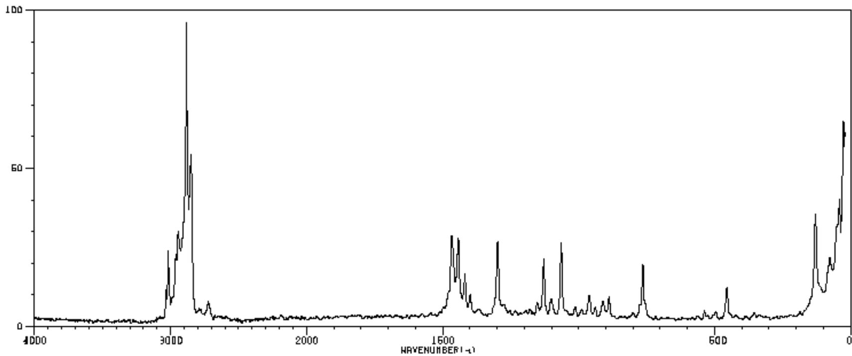
**Figure S5.** Raman spectrum of hexadecyltrimethylammonium bromide collected using Bruker Optics MultiRAM Stand Alone FT-Raman Spectrometer
