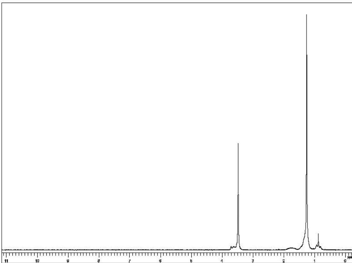
**Figure S3.**  $^1\text{H}$  NMR spectrum of hexadecyltrimethylammonium bromide obtained at 90 MHz using a JEOL FX-90Q; sample was dissolved in chloroform-d and referenced against tetramethylsilane (TMS) standard
