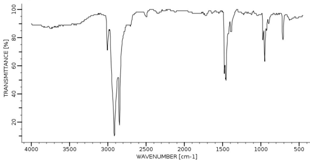
**Figure S1.** FT-IR spectrum of hexadecyltrimethylammonium bromide taken in a KBr pellet using a Nicolet Magna-IR 750 Spectrometer Series II
