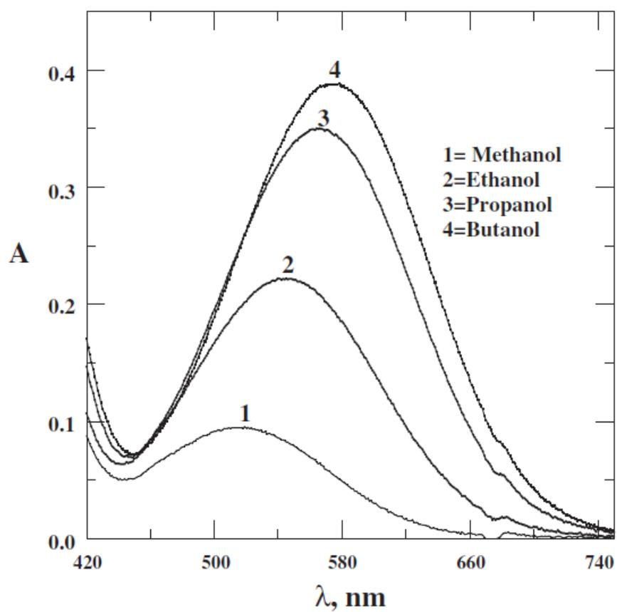
**Figure S2.** UV-Vis spectrum of hexadecyltrimethylammonium bromide with different solvents and their effects; spectrum collected using PerkinElmer LAMBDA XLS+ UV/Vis Spectrophotometer
