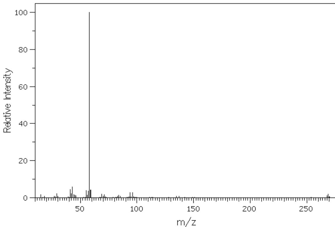
**Figure S6.** Mass spectrum of hexadecyltrimethylammonium bromide obtained using a PerkinElmer 300X NexION Quadrupole Inductively Coupled Plasma Mass Spectrometer (Q-ICP-MS) with a cyclonic spray chamber sample introduction system; samples were stabilized in concentrated nitric acid and diluted to 10 mL with 18.2 MΩ H<sub>2</sub>O
