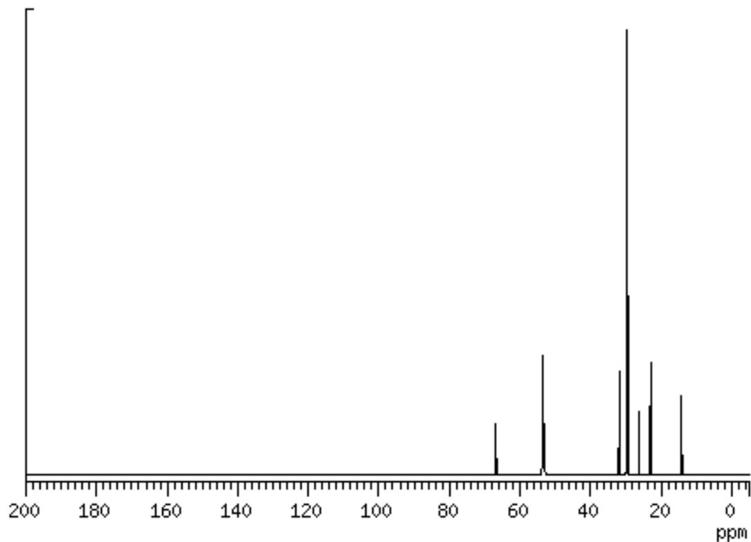
**Figure S4.**  $^{13}\text{C}$  NMR spectrum of hexadecyltrimethylammonium bromide obtained using a Varian CFT-20 instrument; sample was dissolved in chloroform-d and referenced against tetramethylsilane (TMS) standard
