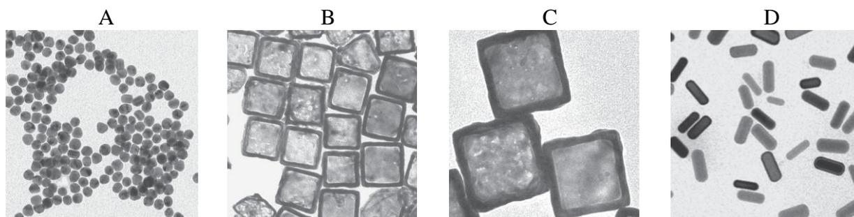
**Figure 6.** TMS Microscope Images of Gold Nanoparticles Following a Manufacturing Process with Hexadecyltrimethylammonium Bromide (HTAB); A-C Show Various Morphologies in Different Aspect Ratios while D Shows the Common Nanorod Morphology
