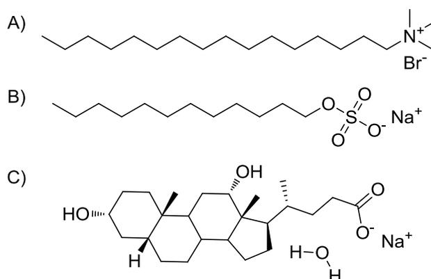
**Scheme 1.** Structures of a) Hexadecyltrimethylammonium Bromide (HTAB) and Other Commonly Used Detergents in Biological Sciences – b) Sodium Dodecyl Sulfate (SDS) and c) Sodium Deoxycholate Monohydrate (SDM).
