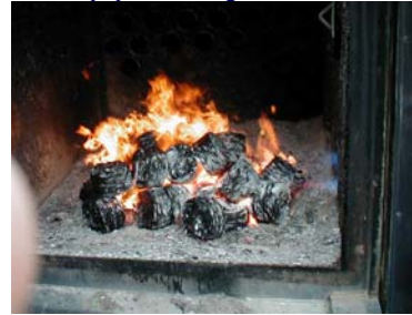
Paper logs used as fuel in the outdoor hot water furnace at MU Agronomy Research Center
